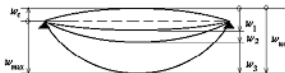
Figure A1.1 - Definitions of vertical deflections
